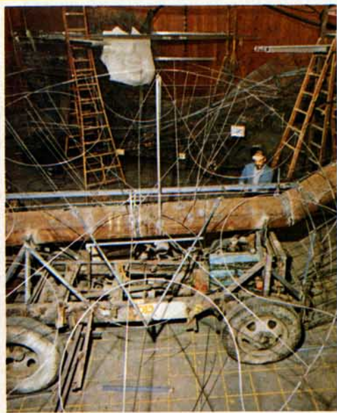
November 15 —Worker sprayed plastic foam onto papier-mache to hold flower viles in place. Should have been sprayed on chicken wire. Mess. We start over.
